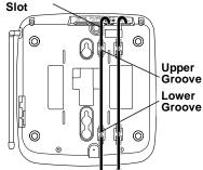
Align the keyhole slots with the mounting screws and slide the base downward to secure it.
